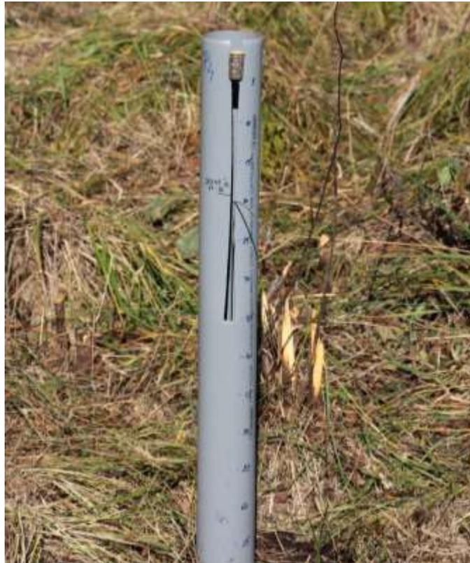
Photo 8- Piezometer installed in the site ROSCI0112 *Mlaca Tătarilor*
