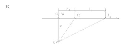
The slant distance d to the PCPA defines the data to be read from the Noise-Power-Distance(NPD)-curves; it defines also the elevation angle. The distance in the horizontal plane from the calculation point CP on the ground to the vertical projection of the PCPA defines the lateral distance for the calculation of the lateral attenuation (if relevant).
